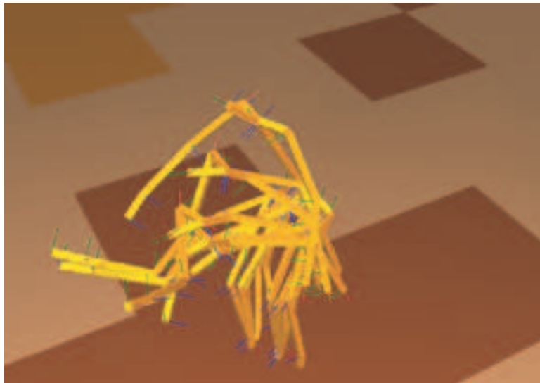
Figure 3.15: Poor motion blend due to dissimilar DOF curves
